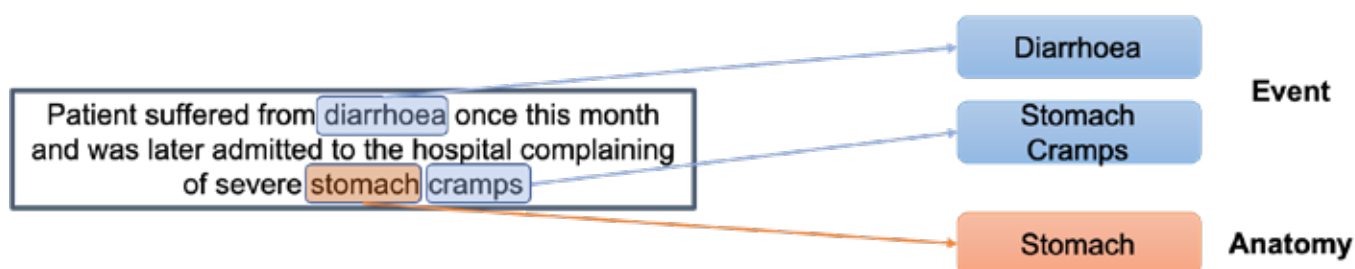
Figure 2: Using Named Entity Recognition (NER) to extract entities from the unstructured text within a patient history
